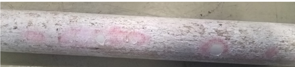
Figure 78 - Bar 4: abrasive wear with red layer
