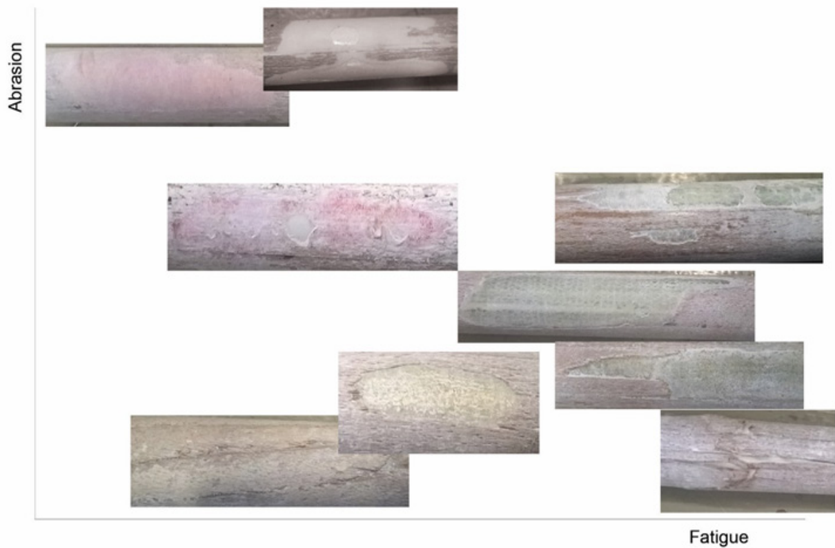
Figure 16 - Graph of abrasion wear vs. surface fatigue. Worn patches of all nine bars are plotted on the graph based on the type of wear.
