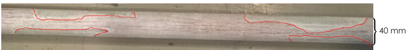
Figure 17 - Worn patches at four places (left and right), marked in red.
