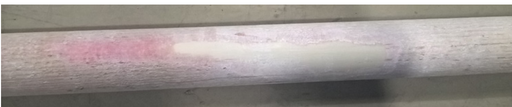
Figure 95 - Bar 8: abrasive wear
