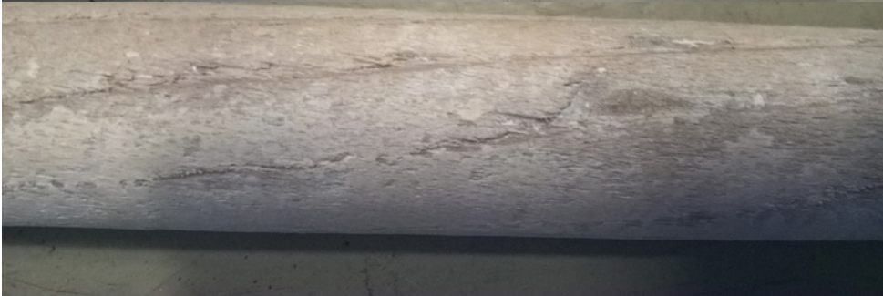
Figure 73 - Bar 3: twisted woodgrain
