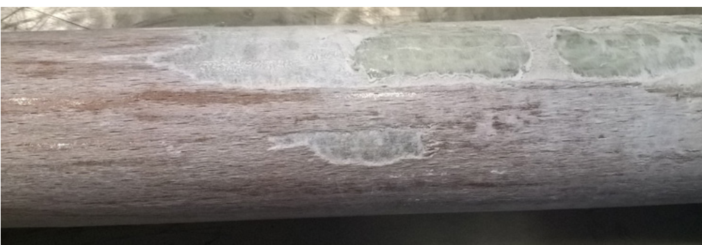
Figure 100 - Bar 9: glue visible
