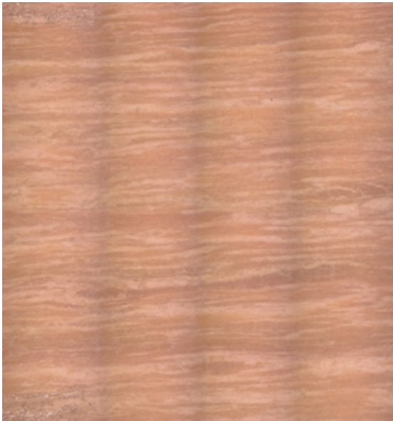
Figure 34 - Photo of a measured surface. The darker stripes show the stitching lines. The white lines look like they are valleys or peaks.
