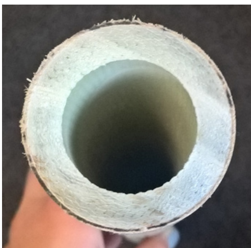
Figure 6 – Cross section of a bar. A core made out of glass fibre, with a thin wood veneer layer around it.
