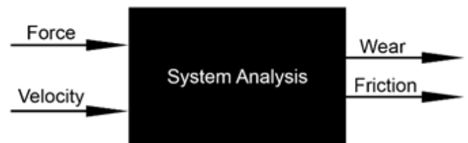
Figure 8 - Black box of system analysis. Input are force and velocity, output is wear and friction.
