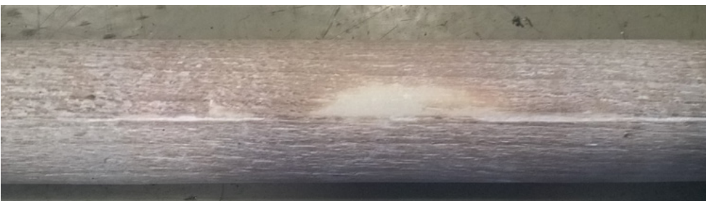
Figure 70 - Bar 2: visible seam
