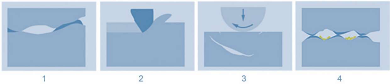
Figure 11 - Wear mechanisms: (1) Adhesive wear; (2) Abrasive wear; (3) Surface fatigue; (4) Tribochemical wear. [38]
