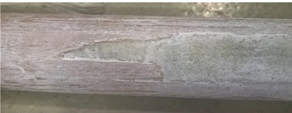
Figure 91 - Bar 7: fatigue and abrasive wear
