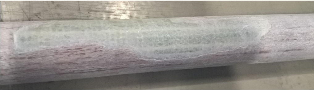
Figure 88 - Bar 6: top right abrasive wear
