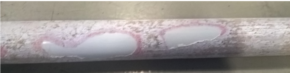
Figure 77 - Bar 4: abrasive wear with red layer
