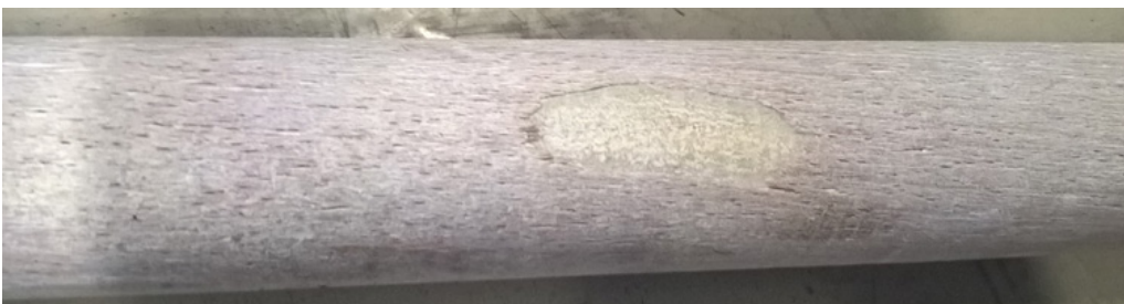
Figure 65 - Bar 1: abrasive wear
