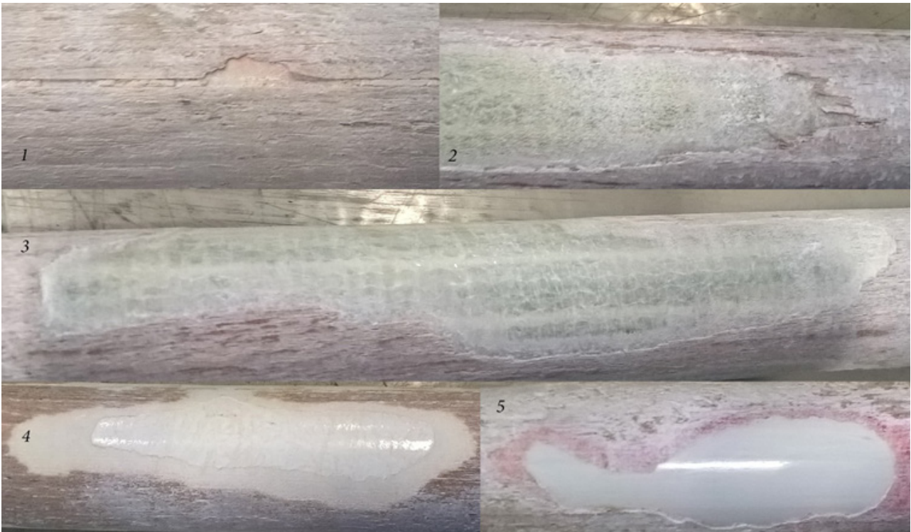
Figure 13 - Worn patches of different bars. (1) Chipped off wood at seam; (2) Splintery at the side and abrasion at the rest of the bar; (3) One big worn patch, with fatigue and abrasive wear; (4) Abrasive wear, with smooth and shiny core; (5) Abrasive wear with red at the edges to show there is wear, and smooth and shiny core.
