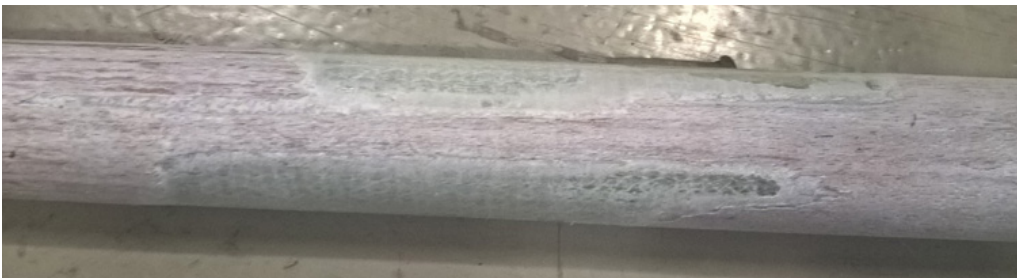
Figure 84 - Bar 6: left side abrasive wear
