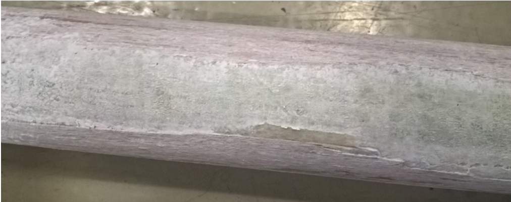
Figure 92 - Bar 7: fatigue and abrasive wear
