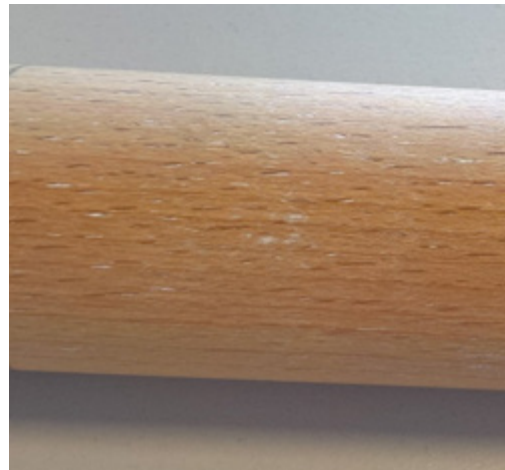
Figure 21 - Sanded bar before testing, part 2, medium sanded down. Tangible noticeable, not visible.
