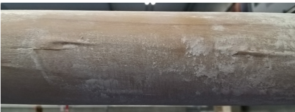
Figure 60 – Wrinkles at the bar appeared after approximately two hours of use.
